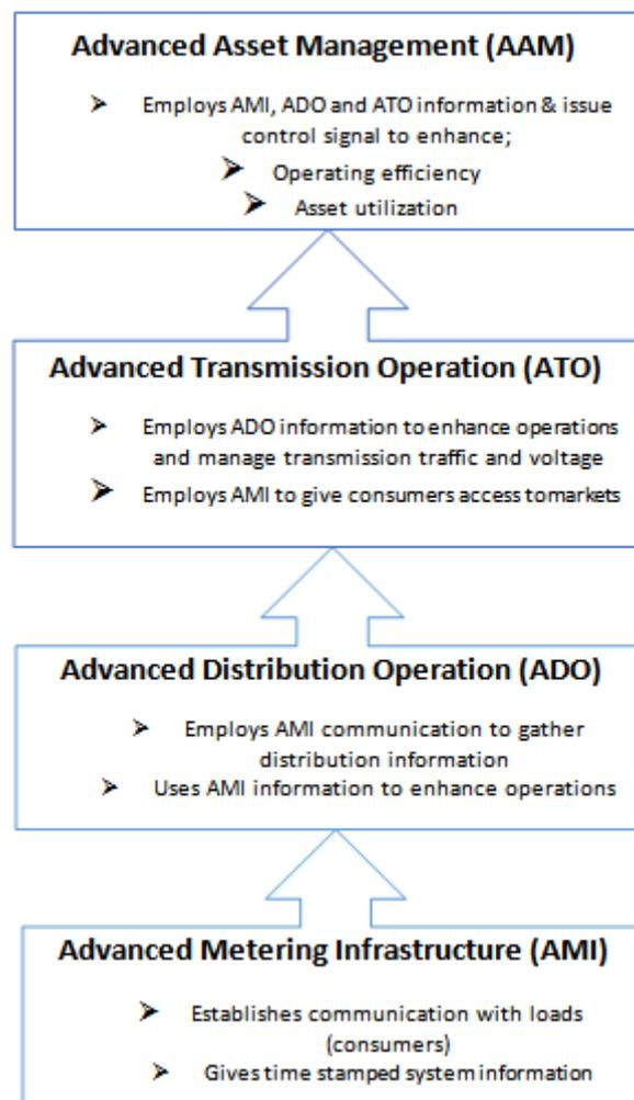
Fig. 1. Smart Grid sub-system sequence overview
