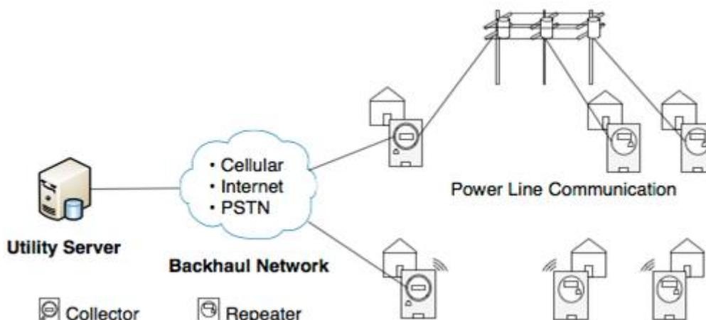
Fig.2: Advanced Metering Infrastructure Security, (SIIS Lab, 2010)
