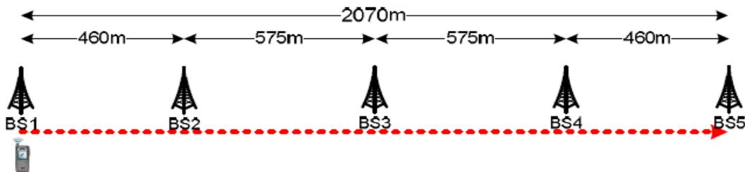
**Figure 3 :**Scenario for evaluation of impact of all techniques on throughput
