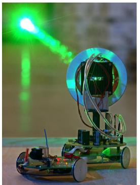
Figure 5: EADS developed, fully laser powered autonomous rover. (Source: EADS)) [10][11]
