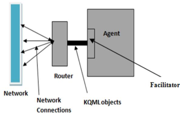
**Fig. 8** - Router provides single interface to the network. It acts both as a client and a server and handles multiple simultaneous connections.
