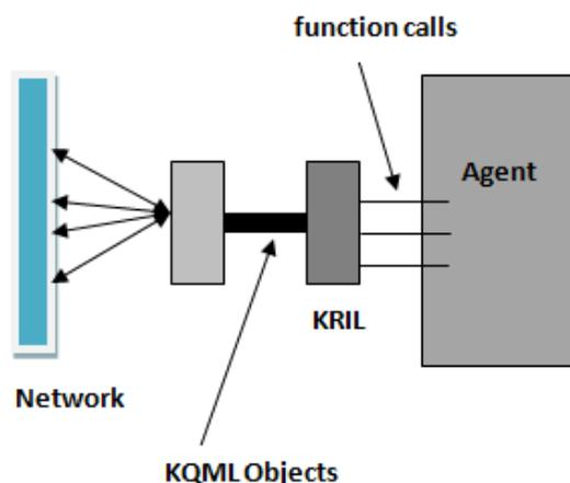
**Fig. 9** - KRIL providing programming interface between the application and the router.
