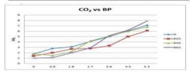
The variation of carbon dioxide with load. The carbon dioxide emission of some were in slightly reduced to mineral diesel as shown in Figure 8. The CO<sub>2</sub> emission decrease with increase in Ester on content in diesel emission were found to be close to diesel emission in case of B40 blend.
