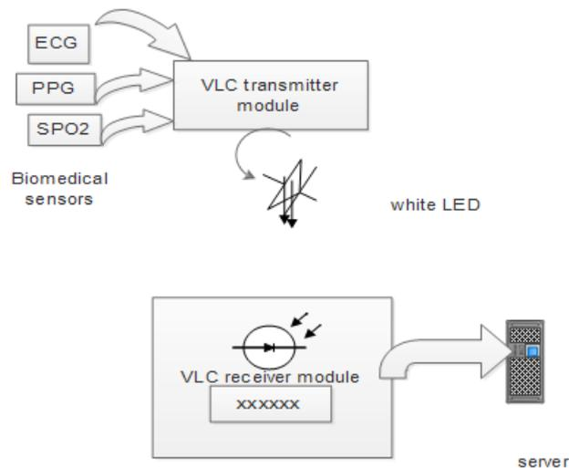
**Fig2.** Experimental setup for indoor VLC system
