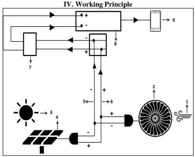
Figure 2: Network line arrangement of non-conventional energy generated unit.
