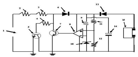
Figure 3: Battery charger processing circuit through solar energy.
