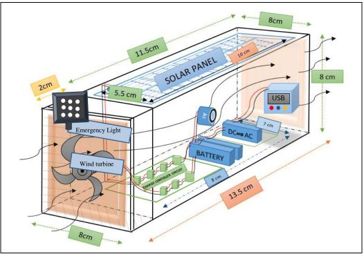
Figure 1: - Sketch showing the conceptual idea behind prototype model
