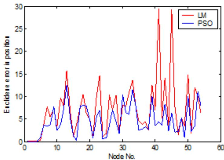
Fig5: Radial error in result shown for position estimation by LM and PSO.
