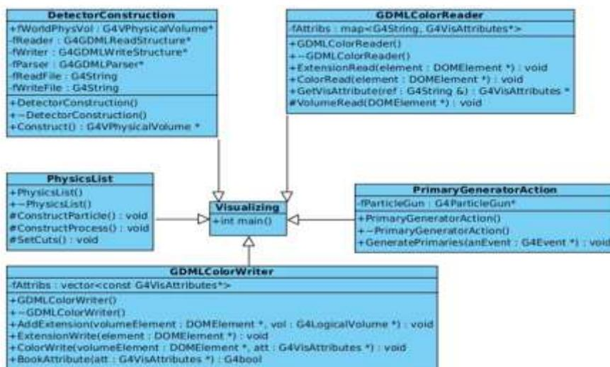
**Fig 1** UML diagram generated from C++ code source of visualizing Geant4 application.
