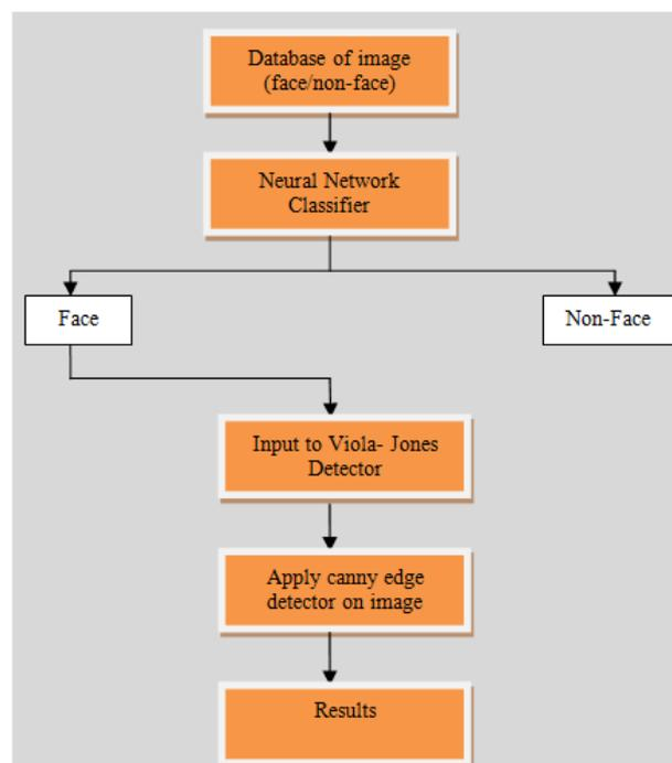
Fig .1: Block Diagram of Face Detection Approach
