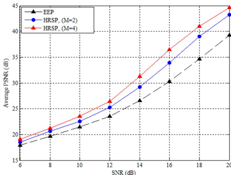
Fig. 2: PSNR performance of HRSP with different numbers of relays.
