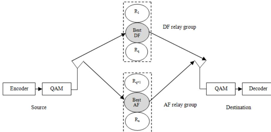
Fig. 1: The proposed Hybrid Relay Selection.
