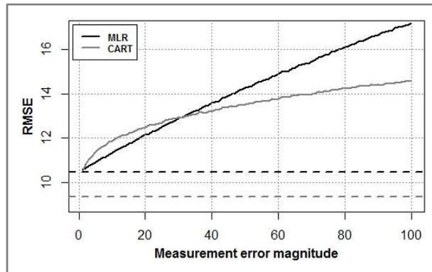
**Figure 3:** Mean RMSE of MLR and CART obtained from data affected by random measurement errors (solid lines) and RMSE values of MLR and CART from data free of error (dashed lines), against error magnitude.
