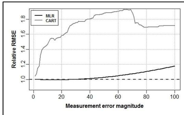
**Figure 7:** RMSE of MLR and CART from data with systematic measurement errors relative to the RMSE obtained from data free of errors, against the error magnitude.
