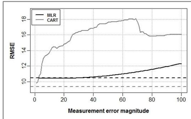
**Figure 6:** Mean RMSE of MLR and CART obtained from data affected by systematic measurement errors (solid lines) and RMSE values of MLR and CART from data free of error (dashed lines), against error magnitude.
