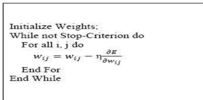
Figure 3: Pseudo code of back propagation algorithm
