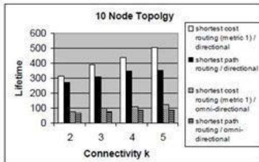
**Fig. 1.** Performance comparison (in terms of network lifetime) of four different schemes, applied to networks consisting of 10 nodes.
