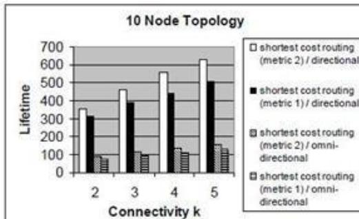
**Fig. 2.** Performance comparison (in terms of network lifetime) of our two metrics used for shortest cost routing, applied to networks consisting of 10 nodes.
