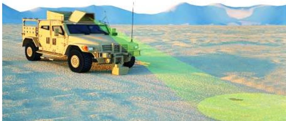
Figure 7: using laser device in the military vehicle's in order to detect the IEDs and other weapons using the laser sample technique
