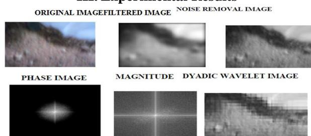
The original image of the soil which is captured by the Logitech Quickcam. The filtered image is the gray scale image which is transformed from the original image in order to point out the noise in the image. The phase image of the soil acquired during removal of noise from the soil. The magnitude image of the soil acquired during removal of noise from the soil. The dyadic wavelet transform occurred during wavelet processing can easily segment RGB color band.
