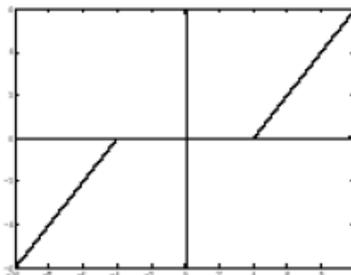
Fig 4: Soft thresholding
