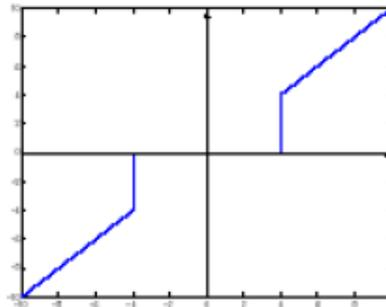
Fig 3: Hard thresholding
