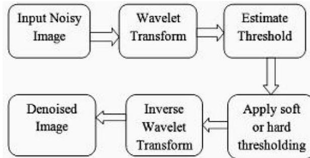
Fig 2: Proposed wavelet based Thresholding
