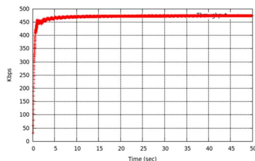
Fig.1. Instantaneous throughput of UDP- separately Fig.2. Instantaneous throughput of TCP- separately
