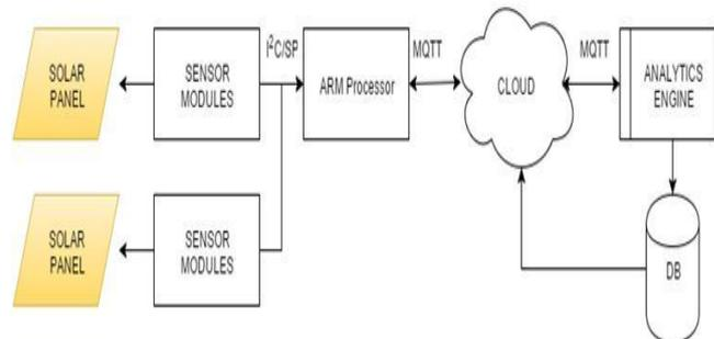
**Figure 1:** Data Acquisition Architecture
