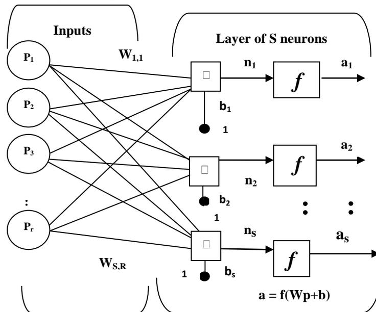
Fig. 2: Multi-Layer Perceptron Architecture
