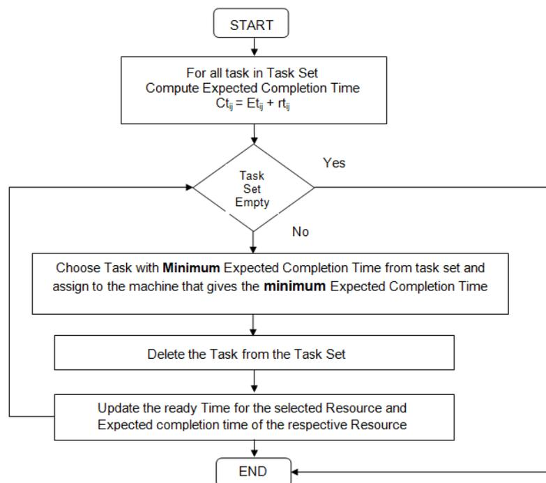
**Fig 3:** Flow Chart of Min-Min Algorithm
