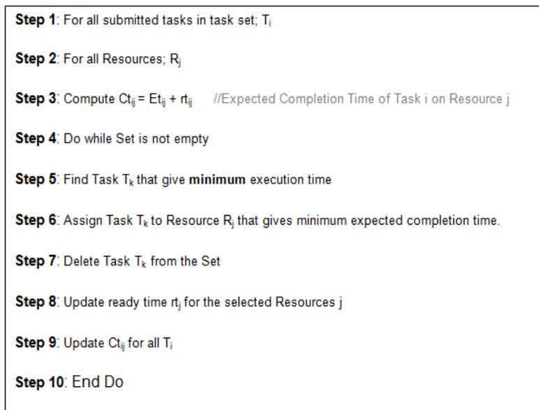
**Fig 2:** Pseudo code of Min-Min Algorithm
