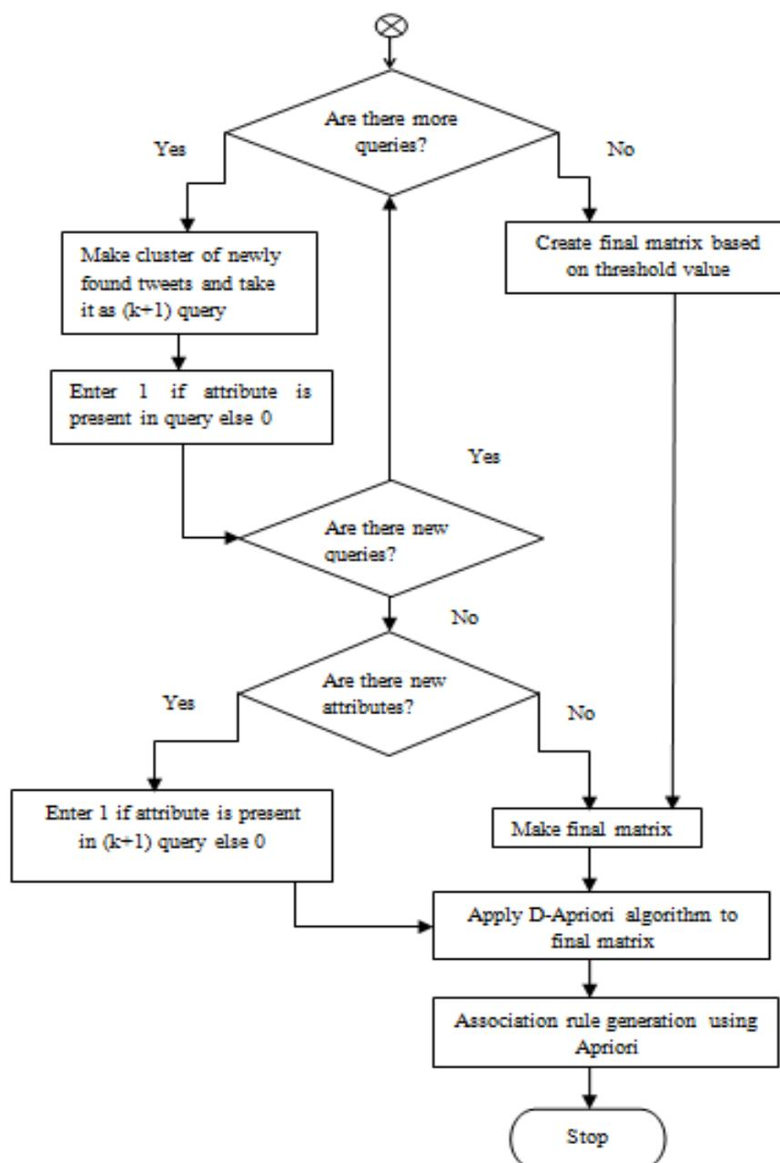
Fig. 1: Flow of k-D-Apriori algorithm
