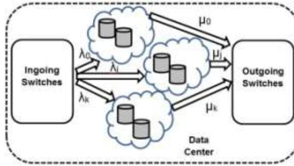
**FIG2.**The proposed delay model using K private clouds to provide a cost-effective cloud system.
