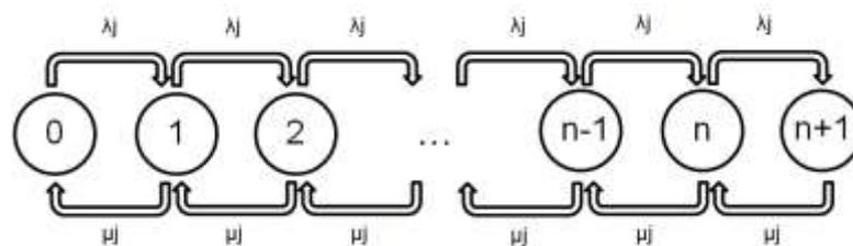
**FIG3.**State diagram for the proposed model.
