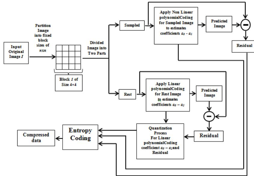
Figure 1- The proposed source coding of compression system.
