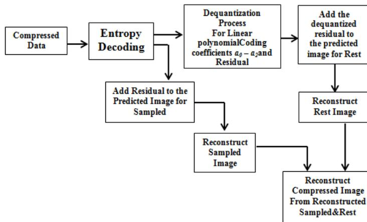
Figure 2- The proposed source decoding of compression system.
