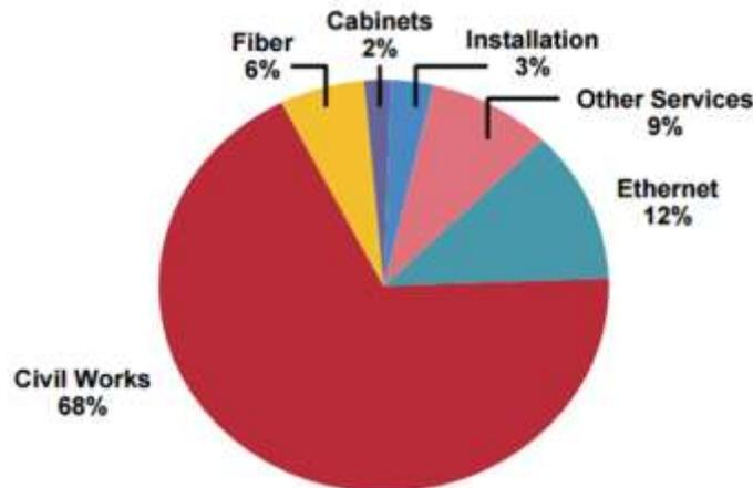
Figure 20. FTTH cost breakdown
