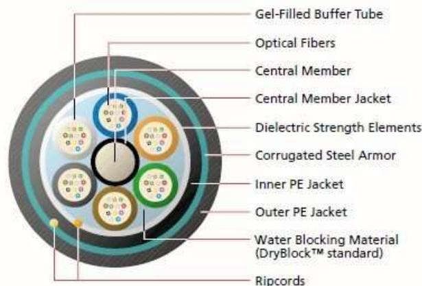
Figure 4. Fiber optic cable
