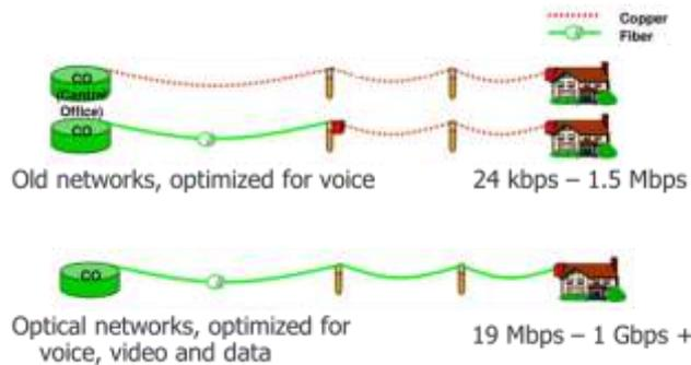
Figure 12. Comparing FTTH and copper network
