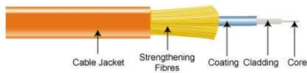
Figure 1. Fiber Optic Cable
