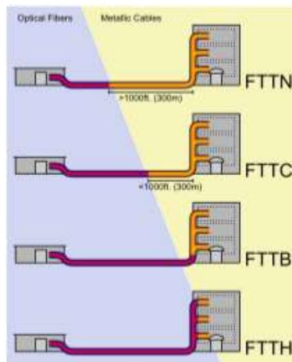
Figure 13. Fiber To The x (FTTx)
