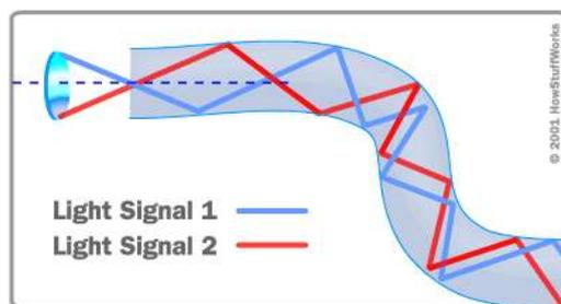
Figure 2. Signal transferring inside fiber
