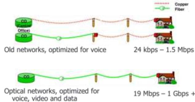
Figure 12. Comparing FTTH and copper network
