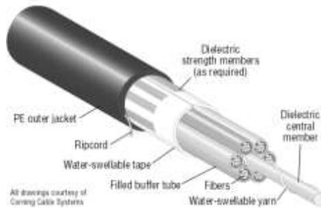
**Figure 8.** Loose Tube Cable Structure
