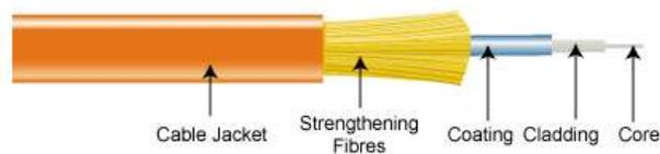
Figure 1. Fiber Optic Cable
