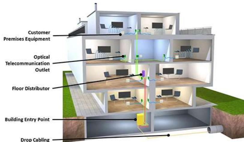
**Figure 17.** Design of basic fiber in the home network
