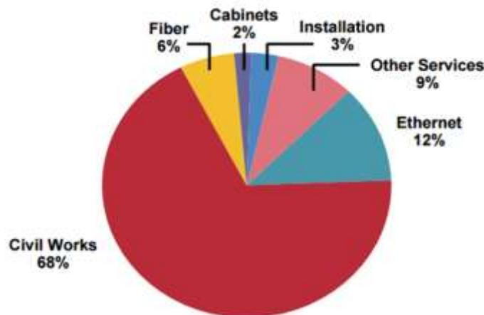
Figure 20. FTTH cost breakdown
