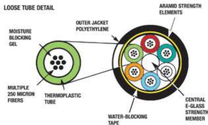
**Figure 7.** Cross-section of loose tube cable
