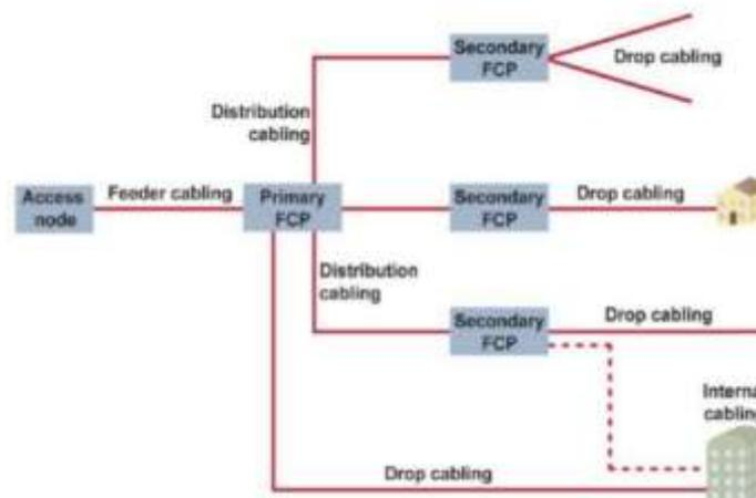
**Figure 16.** Main elements in a FTTH network infrastructure
