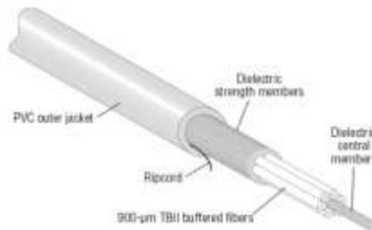
**Figure 10.** Tight Buffer Cable Structure
