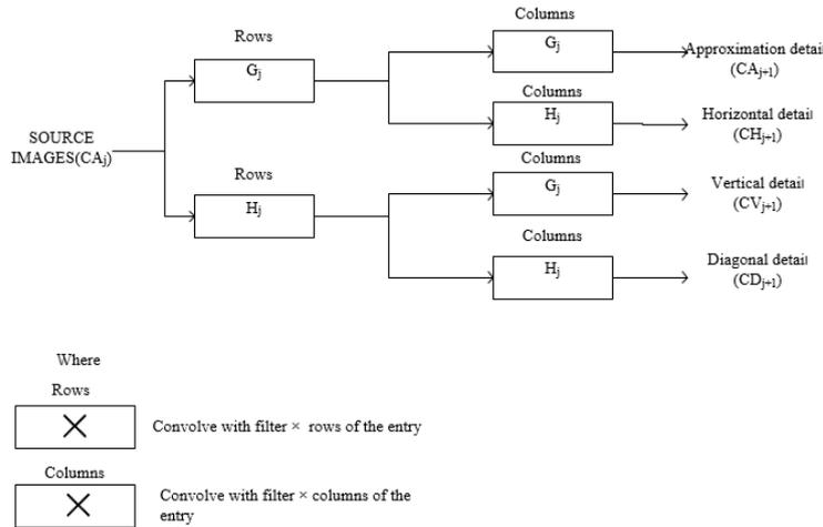
Figure 1 Decomposition steps for two dimensional SWT
