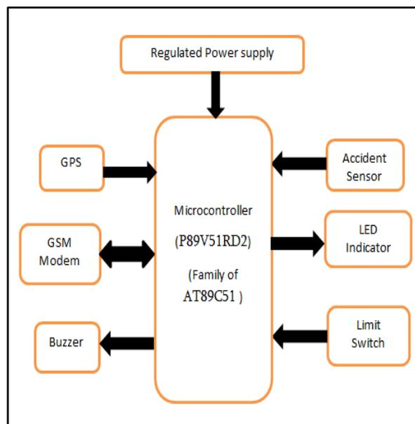
Fig.1(Vehicle Security Block diagram)
