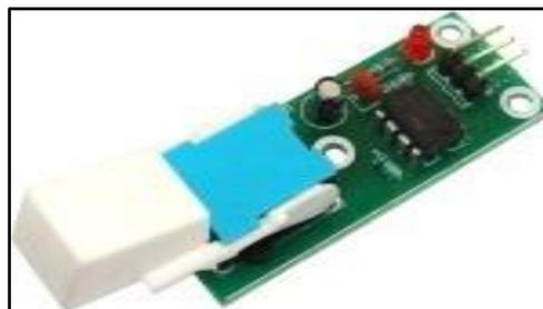
**Fig.6** (Accident Sensor)
