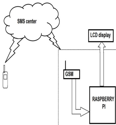
**Figure 3: Architecture of proposed system**
