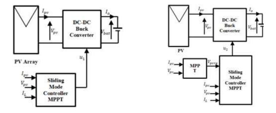
Figure 1. Control scheme with sliding mode Figure 2. Control scheme with sliding mode controller MPPT controller and MPPT algorithm
