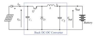
Figure 6. Scheme of the DC-DC buck converter
