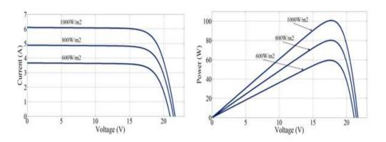
a) (b) **Figure 4.** (a) Current–voltage and (b) Power–voltage curves of PV array at 25°C
