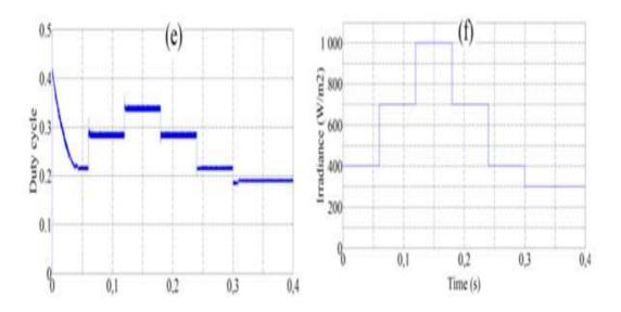
**Figure 8.** (a-c) Respectively voltage, current and power of PV array, (d) load voltage (e) duty cycle of buck control and (f) irradiance profil using SMC P&O MPPT algorithm
