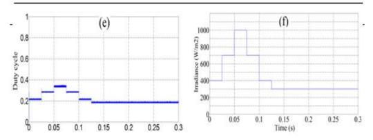
Figure 7. (e) Duty cycle of buck control and (f) irradiance profile using SMC MPPT (continue)
