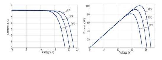
(a) (b) Figure 5. (a) Current–voltage and (b) Power–voltage curves of PV array at 1000 W/m<sup>2</sup>
