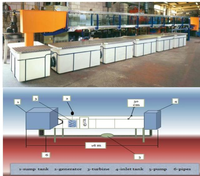
Fig.2. Photo and schematic diagram of Experimental test rig.
