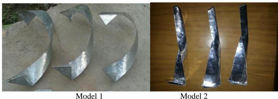
Fig.3. The blade of tow model of turbine. And also it is designed piece circular diameter of 15cm in order to connect the three blades. The final shape of turbine as shown figure (4).
