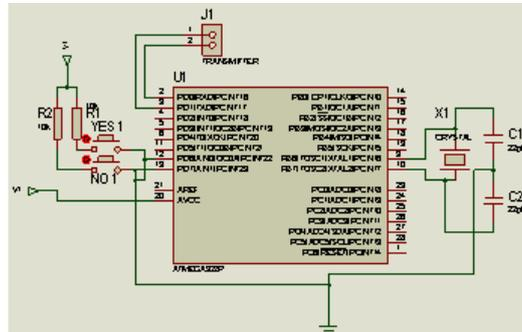
Figure 3. Circuit Diagram of the Input Unit (The keypad)
