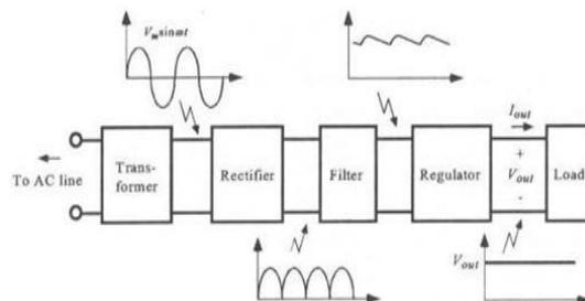
Figure 2. Complete Block diagram of power supply
