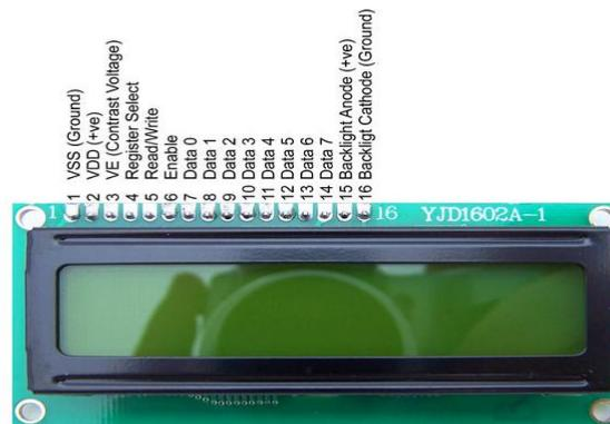
Figure 4. A Liquid Crystal Display (LCD)
