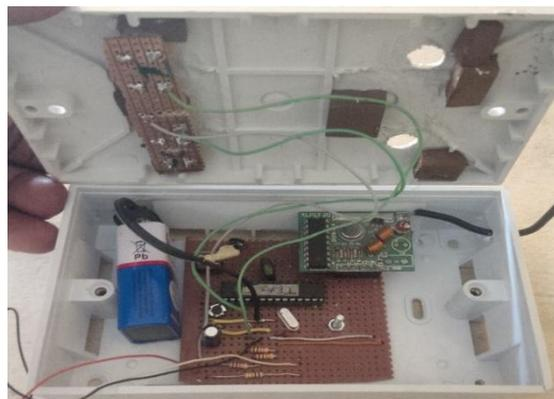
Plate 3. The output/ keypad unit design (the inside view)
