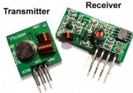
Figure 6. Radio-Frequency (RF) Link: Transmitter/Receiver modules
