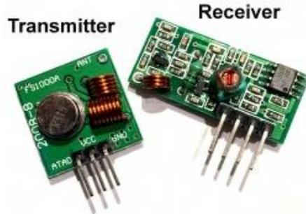
Figure 6. Radio-Frequency (RF) Link: Transmitter/Receiver modules
