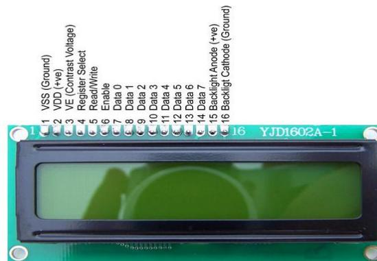
Figure 4. A Liquid Crystal Display (LCD)
