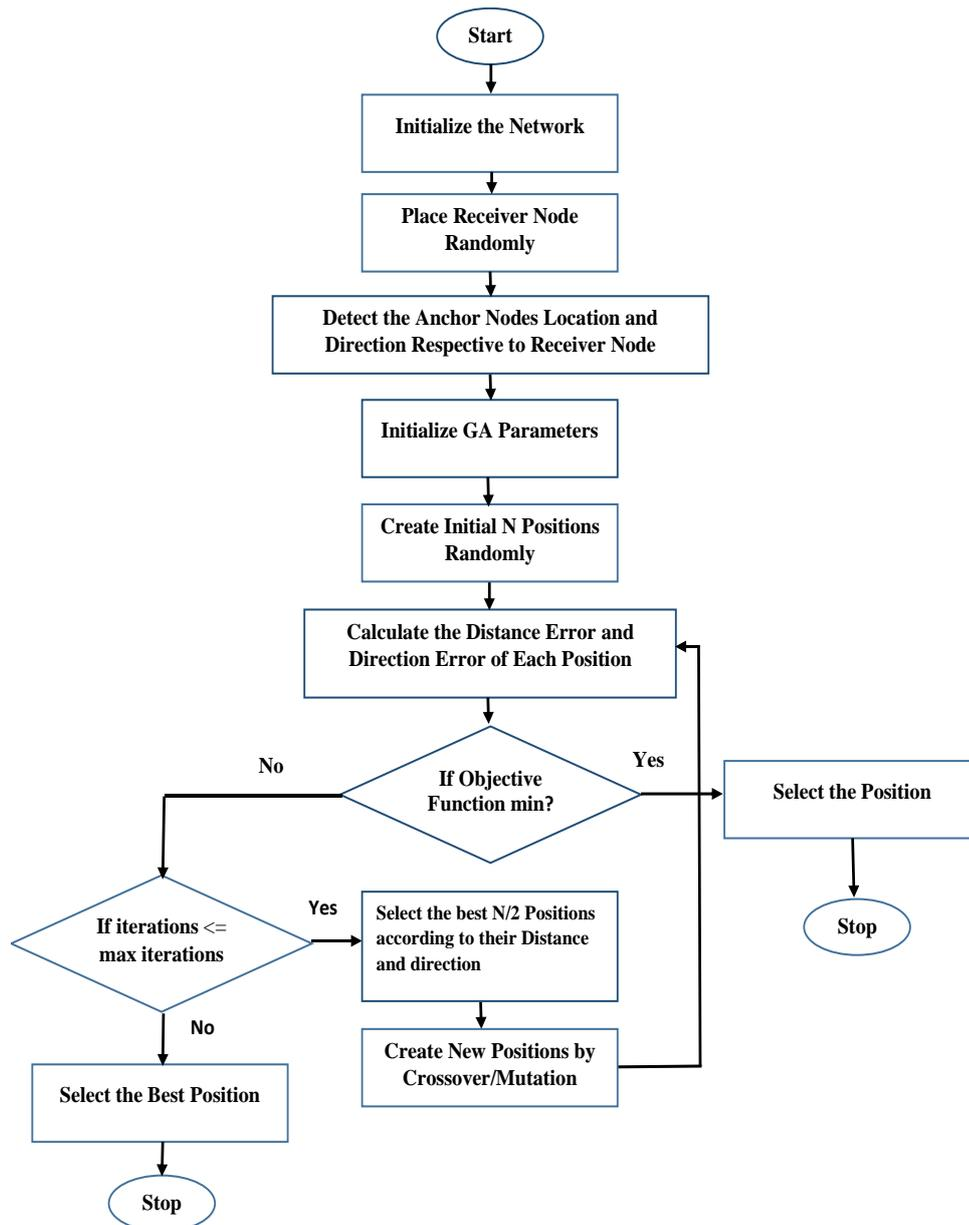
Fig- Flow Chart For Proposed Methodology
