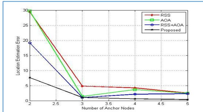
Figure 1: Comparison of the proposed algorithm (RSSI+AOA) with RSSI and AOA for the Location Estimation Error .
