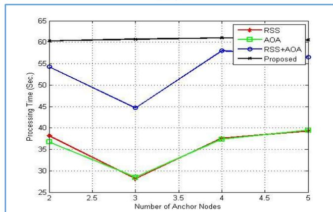
Figure 2: Comparison of the proposed algorithm (RSSI+AOA) with RSSI and AOA for the Location Estimation Time .
