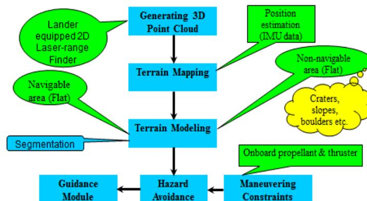
Fig.3. Block diagram of smart landing technology
