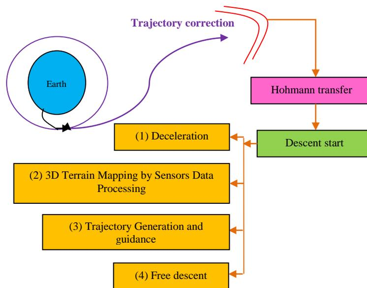
Fig.2. Different sequences of planetary smart landing
