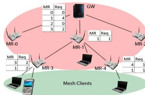
Fig. 2: Distributed requirement tables combined at GW.
