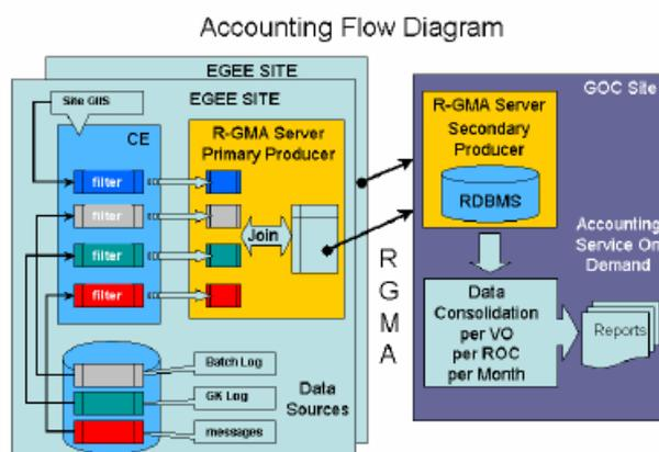
**Figure 8: Accounting flow diagram providing a global overview of the data collection process (APEL), and the web reporting service.**
