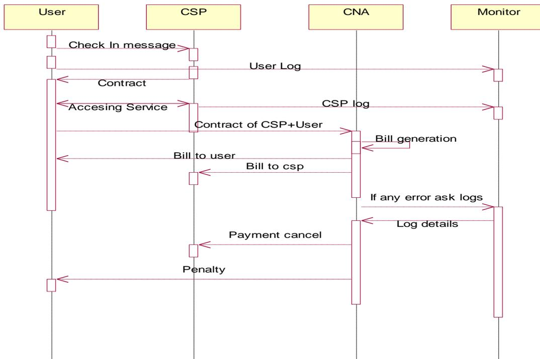
**Figure 17: Sequence diagram for User and CSP**
