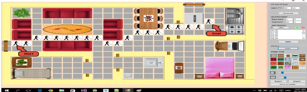
Figure 8 b: Visually impaired/blind people obstacles avoidance using A star algorithm of run 1
