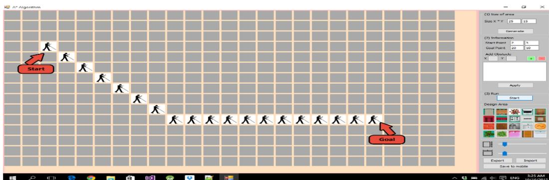
Figure 4 b: Visually impaired/blind people path planning using A star algorithm of run 1
