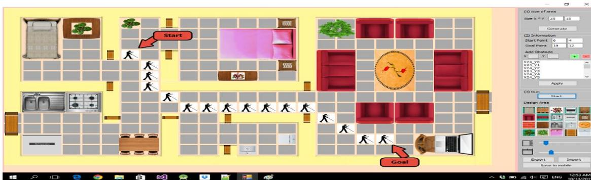
Figure 9 b: Visually impaired/blind people obstacles avoidance using A star algorithm of run 2
