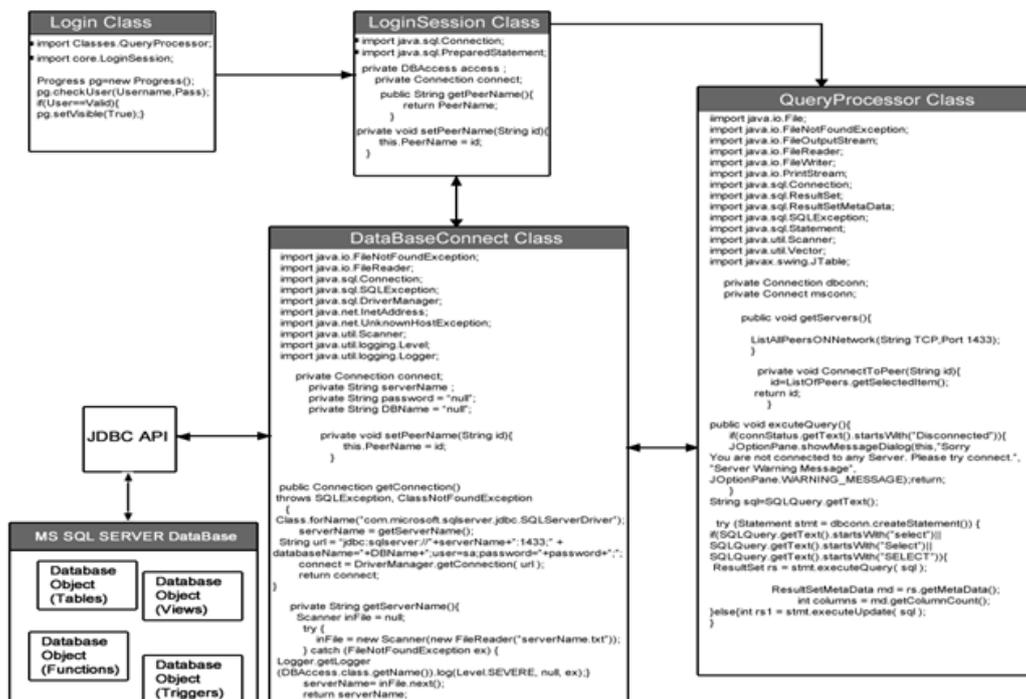
Figure 2: UML Class Diagram of the Proposed System
