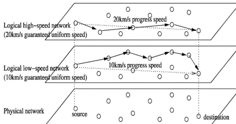
Fig. 3. MMSPEED Architecture [4]
