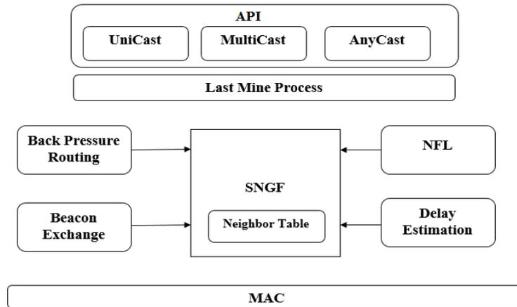
Fig. 2. SPEED Architecture [5]
