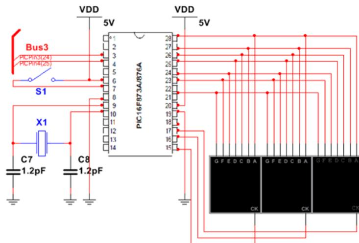
Fig. 5. PIC16F876A and 3 7-Segment Display
