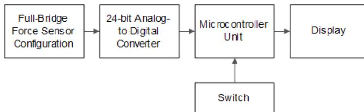
Fig. 1. Force Measurement Instrument Block Diagram
