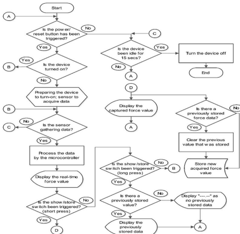
Fig. 6. Force Measurement Instrument Flow Chart
