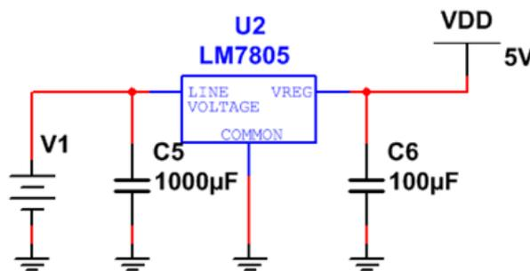
Fig. 4. 5V Power Supply Circuit
