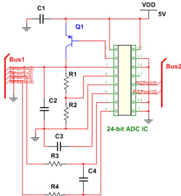
Fig. 3. 24-bit Analog-to-Digital Converter Circuit
