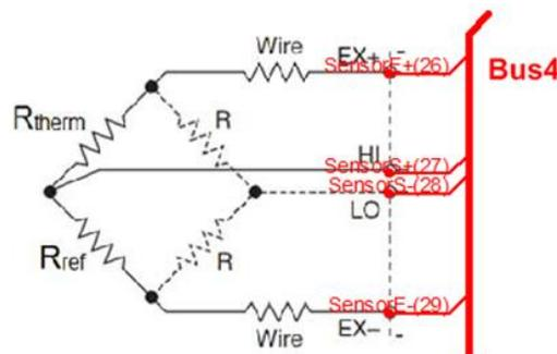
Fig. 2. Full-Bridge Configuration of the Force Sensor
