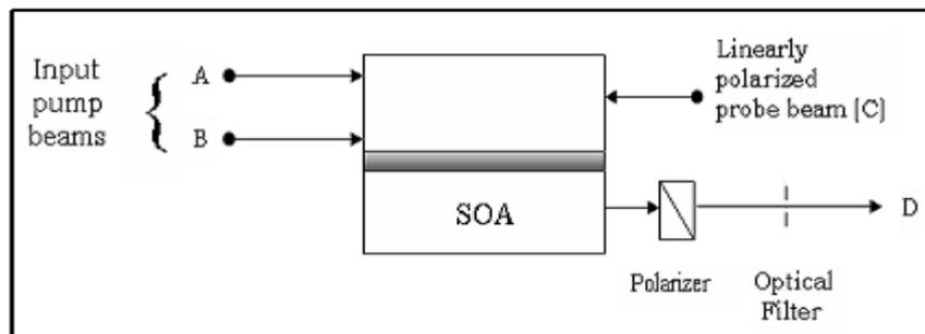
Figure-2: State of polarization rotation of probe beam by SOA
