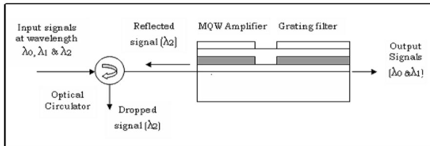
Figure-1: principle of wavelength routing using SOA
