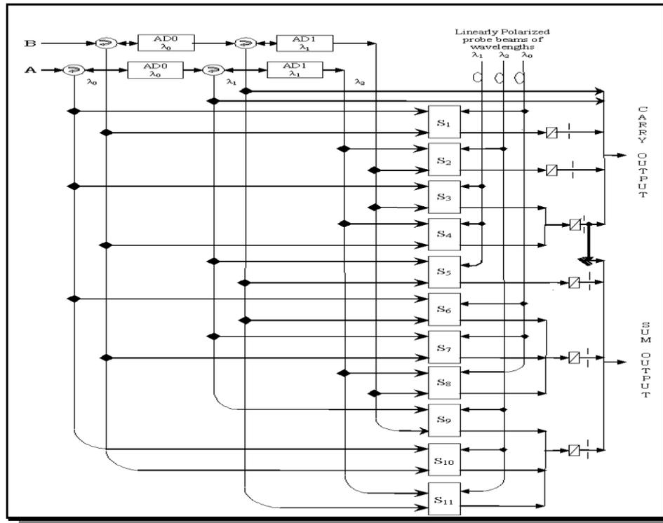
Figure 3: Scheme of the experiment for the Optical Ternary Half Adder
