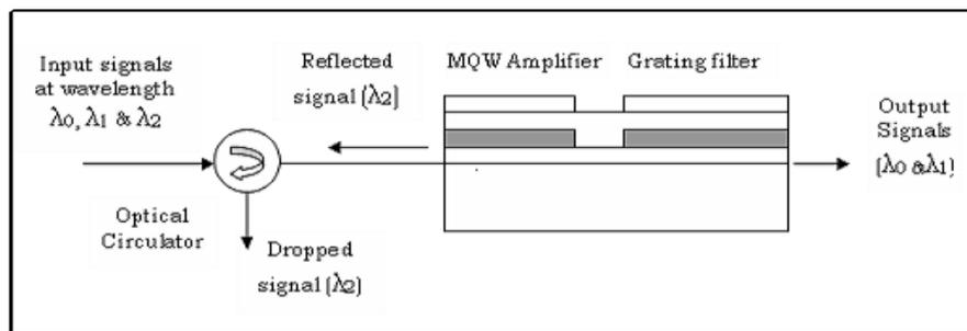
Figure-1: principle of wavelength routing using SOA
