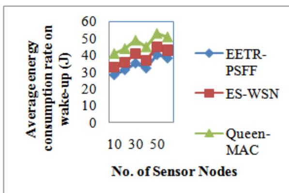
**Figure 4** Effects of average energy consumption rate with respect to varied sensor nodes
