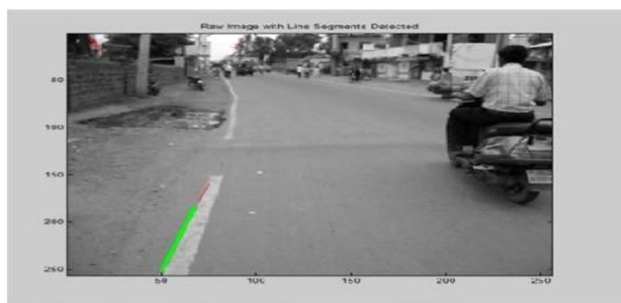
**Fig.9.** Sample result for lane using hough transform in image.
