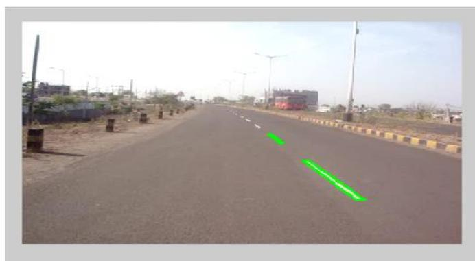
**Fig.11.** Sample result for lane using both hough transform, morphology in video.
