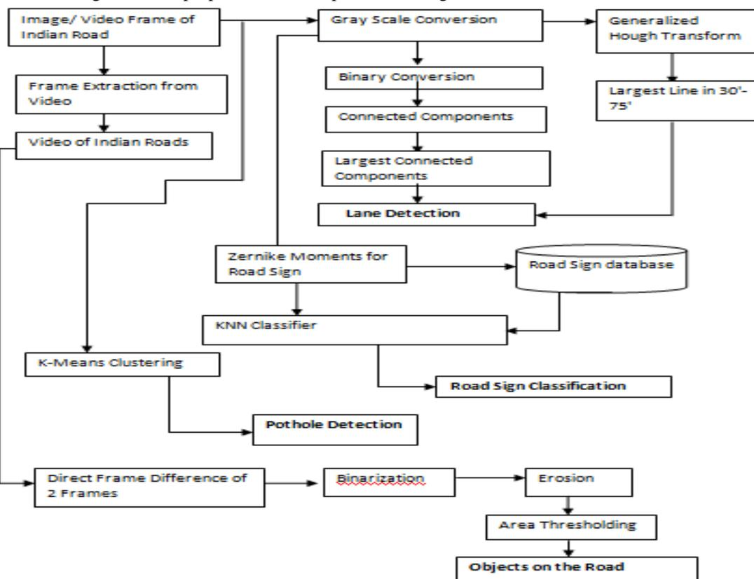
**Fig. 2.** Generalized block diagram of the proposed work.
