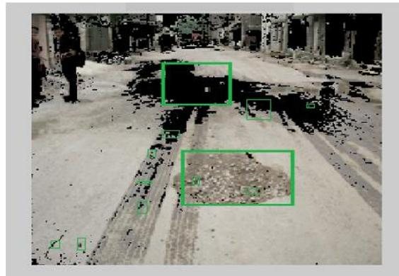
**Fig.13.** Sample result for potholes detection in image.
