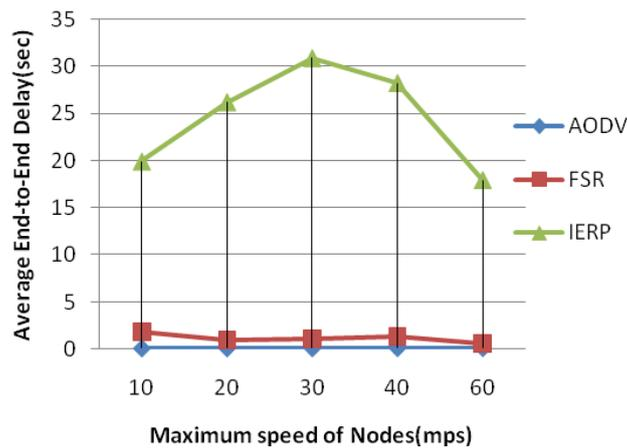
Fig.3 Average end-to-end delay vs. Maximum speed
