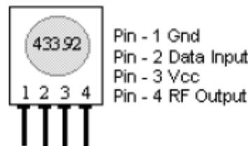
**Figure 6.9: RF Transmitter TWS 434**
