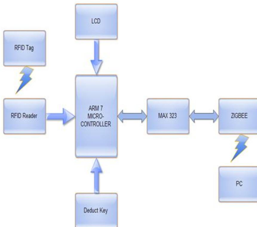
**Fig 4.2: Block Diagram Of System At Trolley**
