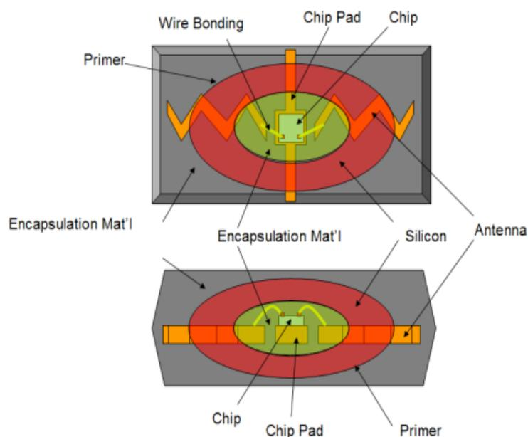
**Fig 6.8: RFID Tag Components**
