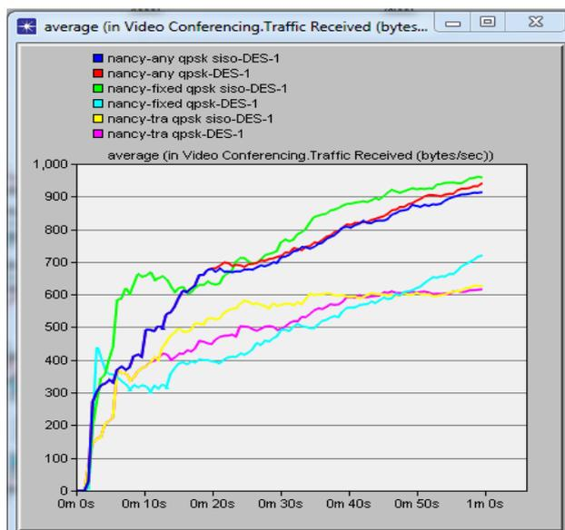
Fig. 3 Traffic received for QPSK
