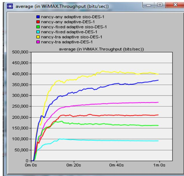
**Fig. 7** Throughput for QPSK
