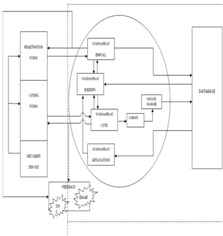
**Figure 2: Model of the Developed E-voting System.**
