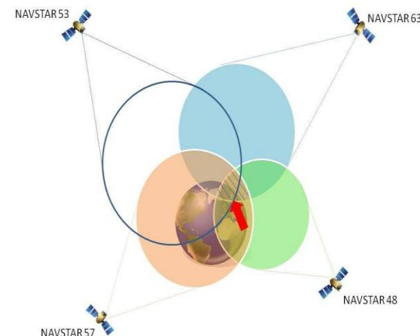
**Figure 1:** Satellites arrangement for accurate GPS positioning [7].
