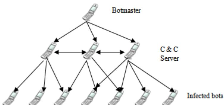
**Figure 1 : Hybrid P2P architecture for C & C Server**
