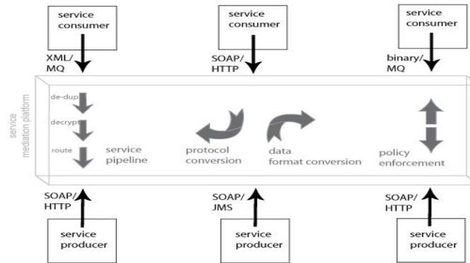
Figure 2: SOAP and XML based mediation
