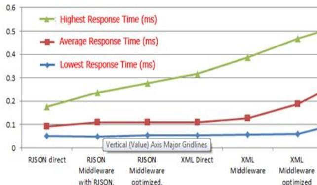
**Figure: 3** Graph of Response Time Comparison
