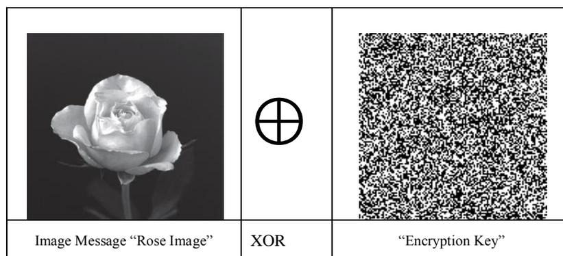
**Figure 3 Send Rose Image Message Encrypted Key by using XOR Operation.**
