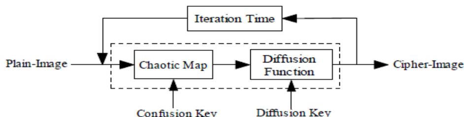
**Figure 2.** The chaos-based image encryption scheme. Here, the plain-image is encrypted into cipher-image through chaotic confusion, diffusion, and repeated iteration.
