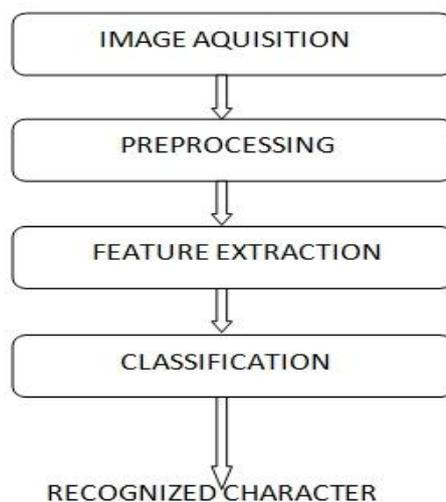
**Fig 2.** Block Diagram of Character Recognition
